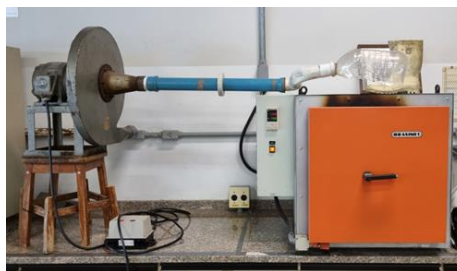
Figure 4 – Muffle and Exhaust fan
