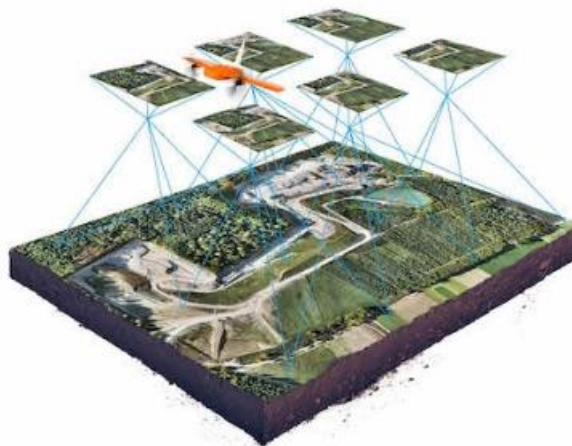
Figure 2 – Topographic Surveys capturing orthophotos using Drone. One way to capture topographic data using drone (Mosaic, 2021)
