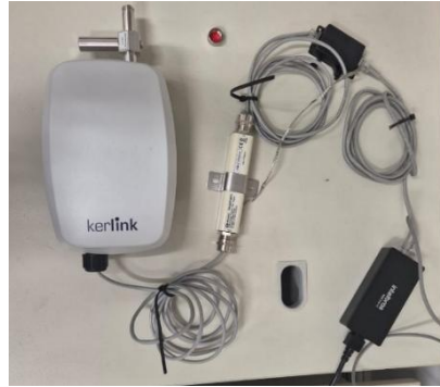
Figure 5 – Gateway Kerlink Wirnet iStation 923 (Assanti et al , 2024).
