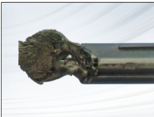
Figura 39 – Cabo ou conector derretido. (Fonte: http://www.ngkeurope.com/en/technology-in-detail/lambda-sensors/diagnosis/defects/ )
